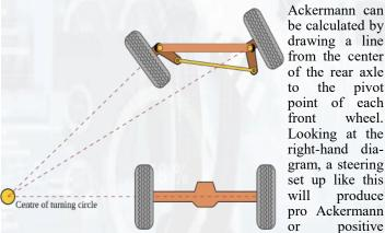
positive Ackermann. If the steering linkage or rack were located in front of the wheel pivot points along the same lines from the rear axle the steering would produce anti-Ackermann as the effect would be reversed and the outside wheel would turn at a greater angle
