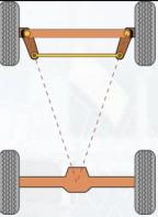
than the inside wheel in a turn. By moving the rack or steering box closer or farther from the centerline of the front axle, either in front of the axle or behind it, the amount of Ackermann or anti- Ackermann can be increased or reduced. Additionally, changes in camber, caster, and static toe can all effect Ackermann. Keep in mind that this the 30,000foot view of this subject. There is much, much more to this when the application is for cars built for specific types of racing and it is differ-
